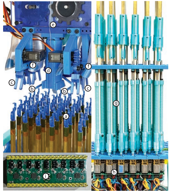
Figure 9: Our proof of concept implementation. It includes a 6x6 bed of needles (a), two sweeping arms used to ease yarn capture (b), two sets of two transfer grippers (c), a compactor (d), a yarn feeder used to control yarn delivery and tension (e) and a set of blowers used to stabilize loop creation (f). Each needle includes two hooks, that are independently actuated using 3D printed lead screws (g), and controlled by geared motors (h). We used a custom designed board (i) to PID control a group of 8 motors each. Our configuration is using 72 motors in total. During printing, the needle assembly is moved whereas the yarn feeder and the transfer tools remain fixed.
